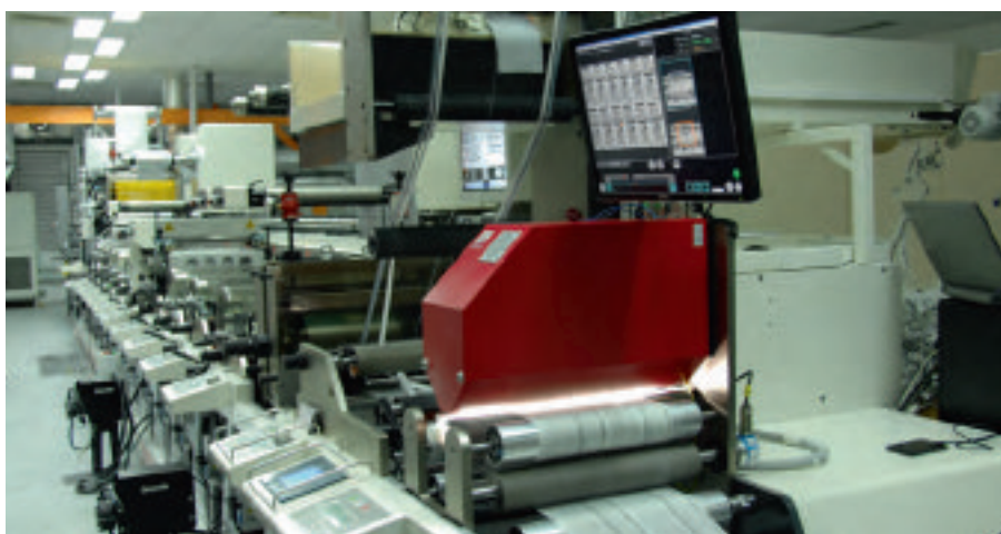
EyeC's 100% inline print control shown on press
